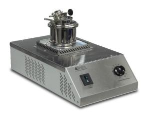
Figure 5: Assembled Tag Closed Cup Flash Point Tester
